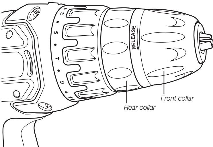
Hold the rear collar with one hand and twist the front collar with the other hand to tighten or undo the chuck.
