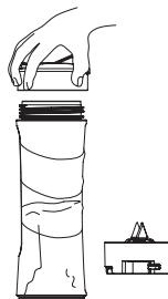
3. Turn the beaker upside down and screw it onto the motor unit (clockwise).
