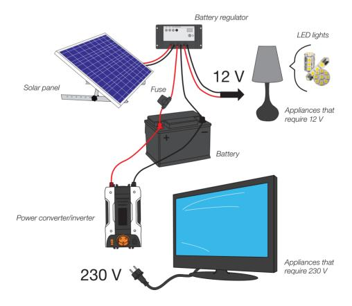
The solar panel must be installed outdoors facing south. The battery regulator and the battery can be installed in a suitable location indoors or outdoors, preferably close to the appliances that will be using the solar power (inverter, lights, TV, etc).
