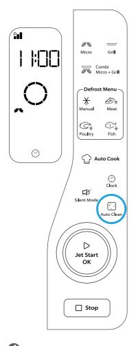
This automatic cleaning cycle will help you to to clean the microwave oven cavity and to remove unpleasant odors.
