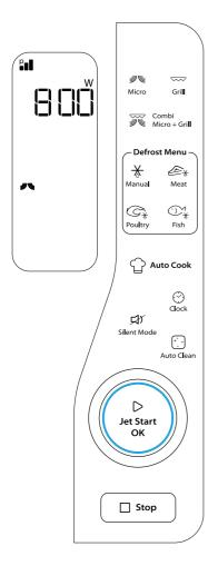
This function allows to start the Microwave function at maximum power for 30 seconds, simply pressing the Jet Start button. It is suggested for quick reheating of food with a high water content such as clear soups, coffee or tea.
