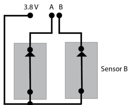
**Figure 3** Two alarm sensors with breaking function
