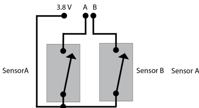
**Figure 2** Two alarm sensors with closing function
