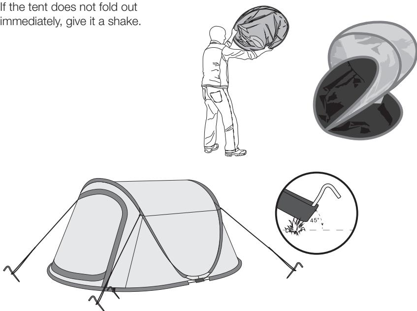
4. Anchor the tent with 4 × tent pegs (7) that are pushed into the ground through the four holes (8) next to the floor tubes on the outside of the tent.
