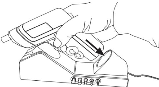
3. Plug the charging cradle into a wall socket. The indicator light (4) comes on when the battery is charging and goes off when the battery is charged (approximately 4–6 hours).
